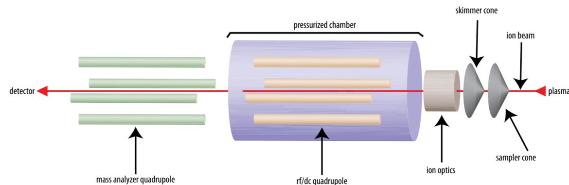
interferences, PerkinElmer's Dynamic Reaction Cell™ (DRC) improves significantly upon conventional analysis by ICP-MS. Located between the ion optics and the mass analyzer vacuum chambers of an ICP-MS instrument, the DRC is an enclosed and positively pressurized chamber with an independent quadrupole that can be configured to nearly eliminate polyatomic spectral interferences.
