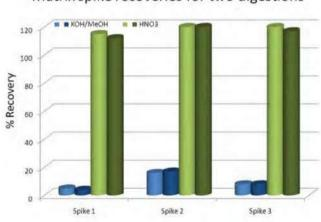
Figure 3a: Three of the samples displayed in Figure 2a were selected for matrix spikes. The matrix spike was digested in duplicate by each method and analyzed with the samples at the default volume. The recovery of the matrix spikes for the KOH/MeOH digestion were all less than 20%, whereas the recovery for the HNO<sub>3</sub> digestion were all greater than 100%.
