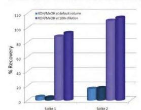
Figure 3b: A matrix spike and matrix spike duplicate were prepared by KOH/MeOH digestion. The digests were analyzed at default volume and at a 100x dilution and were analyzed on the same day. The spike recoveries change drastically from 2-3% at default volume to 88-114% when analyzed at 100x. This demonstrates the level of interference present at default volume.
