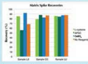
Graph D. Recoveries for matrix spikes on the experimental samples. Sample LS was spiked at 0.5 ng/L, and Samples CC and UJ were each spiked at 0.2 ng/L. The matrix spike prepared with APDC yielded a 58% recovery for Sample LS, below the recovery criteria of 65-135% specified in EPA Method 1630. All other matrix spike recoveries were within the EPA Method 1630 acceptance criteria, though the matrix spike on site LS that was prepared without reagents recovered near the bottom of the acceptance range at 68%.
