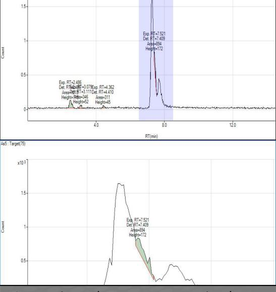
Inexperienced operators may miss that the big peak is due to Nd<sup>++</sup> eluting very close to the As(V) peak. The peak after As(V) is from Sm<sup>++</sup>.
