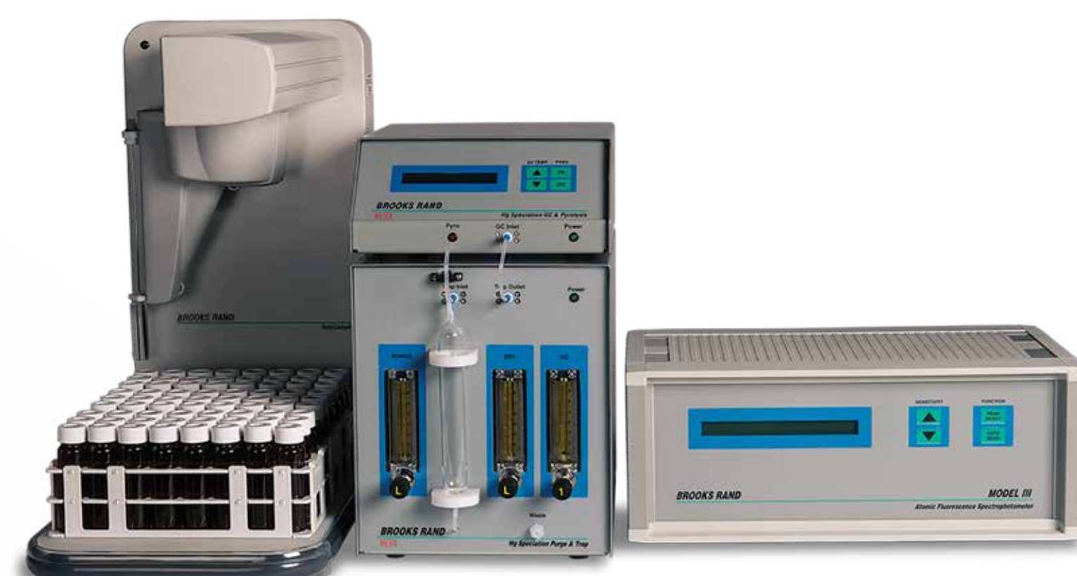
Figure 5. Brooks Rand Instruments MERX-M used for total and dissolved methylmercury analysis. A modification of the MERX-M system was also used for the automated analysis of dimethylmercury by AFS.
