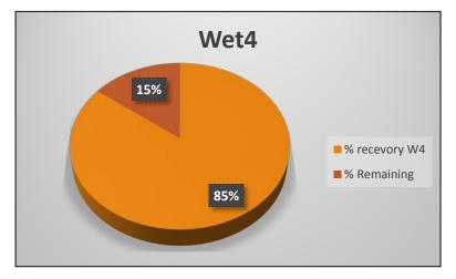
Average recovery = 83%RSD = 2.5%recovery based off Hg<sub>total</sub> added 0.25 mL H<sub>2</sub>O
